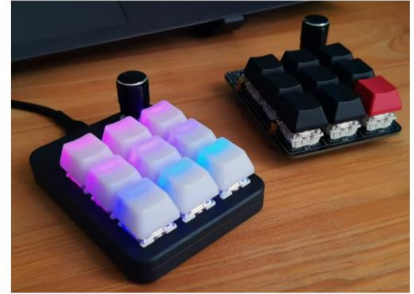
MacroBoard | 9-key hotswap mechanical macropad
